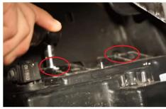
4-8. When you get the fuse joint, you'll also need an extension cable, and 16awg will be enough. The DRL will work just like the real DRL. If you do not want to disturb the fuse connector, you can also splice the yellow wire with the red extension cable in the package to the positive pole of the front position lamp. The DRL only works when the position light is on.
