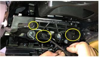
5. Remove the ribbed plastic clip on the side of the fender. After this, you can remove the bracket.
