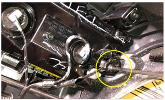
7. Remove the two T20 Torx screws at the top of the OEM DRL.
