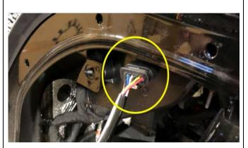
4. Unscrew the three T25 Torx screws on the bracket the bracket behind on the OEM DRL.
