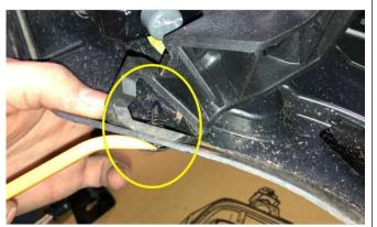
6. Remove the T25 Torx screw holding the side marker in place.
