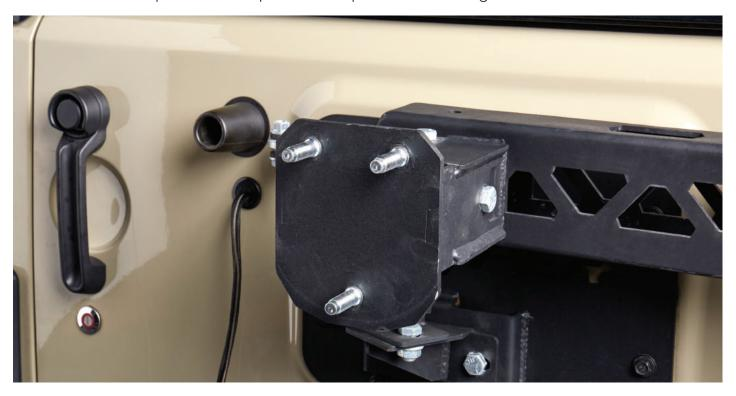
**STEP 2.** Place the Lumen LED 3rd Brake Light over the spare tire carrier studs. Ensure that the wiring harness is located at the 6 o'clock position on the 3rd brake light.
