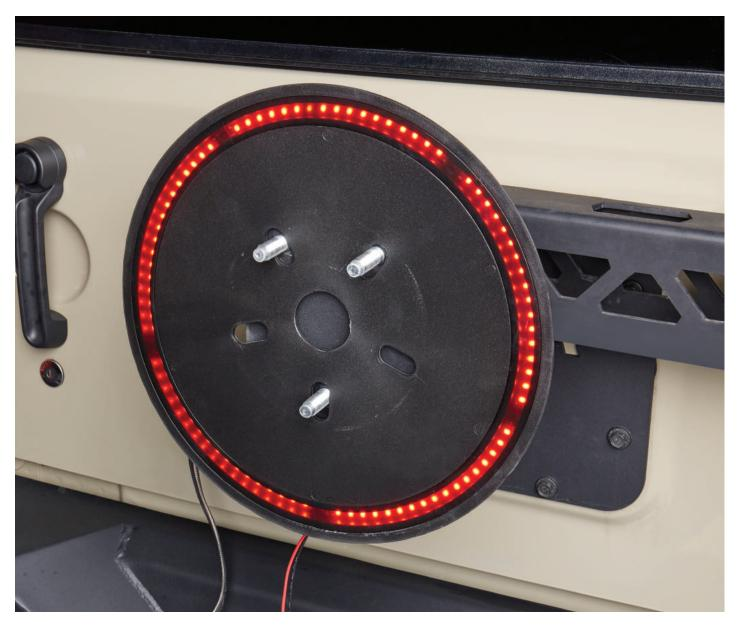
**STEP 8.** Using cable ties, secure the wiring harness to the spare tire carrier free from any moving parts. Carefully open and close the trunk door, make sure the wires do not get pinched or pulled during the operation of the door.
