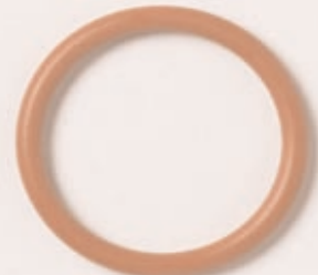
Normal O-Ring Softened and Swollen After Soaking In Seal Swell Product.
