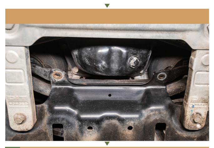
**6** USE A JACK AND PIECE OF WOOD OR A FRIEND TO HELP SUPPORT THE BUMPER GUARD DURING INSTALLATION
