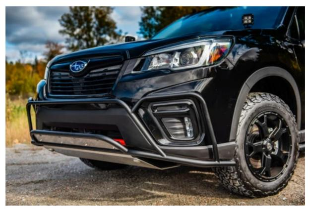
The LP Aventure bumper guard for the 2019-2021 Subaru Forester are manufactured in DOM (Drawn Over Mandrel) steel tube of 1.25" x 0.125" combined with 1" x 0.095". This material is very strong and is often used in the manufacturing of roll cage.
