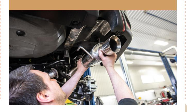
4 USE INCLUDED BOLTS AND GASKET TO BOLT UP AXLE BACK
