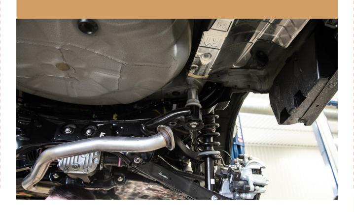
3 INSTALL LACHUTE PERFORMANCE AXLE BACK. WE RECOMMEND SPRAYING THE EXHASUT HANGERS WITH SOME LUBRICANT FIRST
