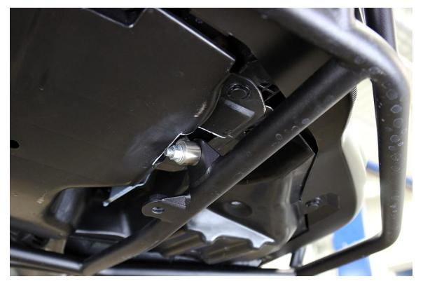
**#7** : Bolt up the rear section of the bumper guard
