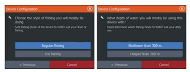
Sonar presets will be adjusted to best suit selection made. All presets can be adjusted at a later date via the sonar page menu, and under settings/sonar.
