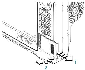
The card reader door should always be shut immediately after inserting or removing a card, in order to prevent possible water ingress.
