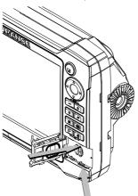
Remove the bezel from the display by first opening the card reader door. Using a fingernail or small flat screwdriver, pull off the bezel at the slotted points immediately above and below the card reader. Pull bezel around keypad forward, till hidden tab at top right can be disengaged by a slight downward pull. Applying a slight twist to top bezel edge will disengage the top left hidden tab. The rest of the bezel should come away easily.
