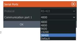
→ **Note:** AIS transponders typically operate at NMEA 0183-HS (high speed), and will require the baud rate to be set to 38,400.
