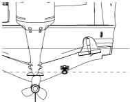
→ **Note:** Ensure the entire bottom surface of the transducer hangs at least 3 mm (1/8th of an inch) lower than the bottom of the hull.
