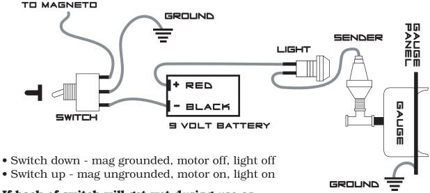
If back of switch will get wet during use or washdown seal it with a good silicone sealer.
