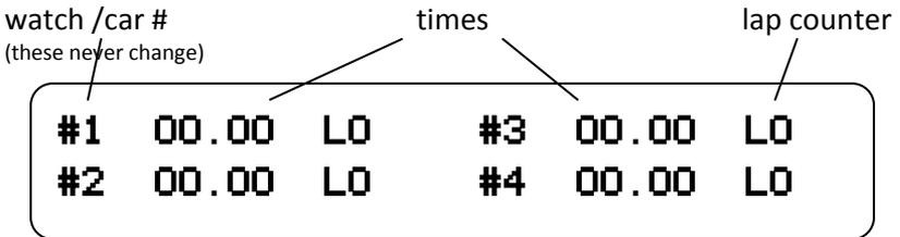
**TO USE THE STOPWATCH FUNCTION:** Use buttons #1 to 4 (pyrometer Memory) for timing. These correspond to #1 to #4 on the display.
