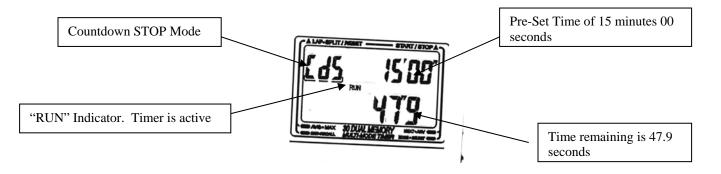
"Time Out". You may stop and restart the CDT by pressing "A". While stopped, the "STOP" indicator will appear. You may restart the timer by pressing "A" or reset to the original preset time by pressing "B".
