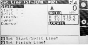
A NOTE about setting your START/STOP line and Segments for lap times: The GPS records your position within 6-10 feet so you should choose a location on the track where you will have the most consistent positioning. Choosing an area where you frequently change your line may result in laps not being recorded.
