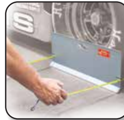
Magnets hold tapes in place during use.
