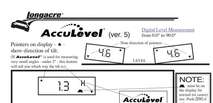
**NOTE:** This Ver. 5 **Acculevel**<sup>™</sup> has 2 modes of operation. 1) In Normal angle measurement mode the display is steady. 2) In Caster Mode the display flashes (and will not measure absolute angles). Push CASTER button to exit Caster mode and go back to Normal angle measurement.
