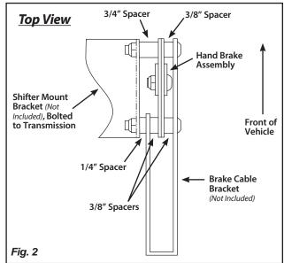
Step 4: Follow the instructions for the Transmount Emergency Brake Cable Kit to connect the emergency brake cables. Adjust the Hand Brake so that there is no slack, but make sure that the brakes are not applied when the Hand Brake is released. Generally, you will want the cables adjusted so that three clicks of the Hand Brake will prevent the vehicle from moving (although your braking system may be different). Your completed installation should look like Fig. 3.
