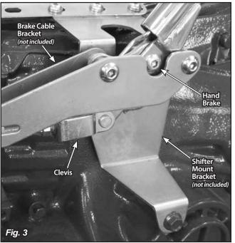
NOTE: To release the Hand Brake, you must pull up slightly on the handle while depressing the release button. Keep the release button depressed while you lower the handle to it's at-rest position.
