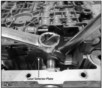
Step 13: AODE and 4R7OW Only: Install the new Lokar flange onto the selector shaft. If using the original selector shaft, use the original nut or bolt to retain the flange. If using the Lokar selector shaft, install the supplied 3/8"-16 x 3/4" lock bolt into the selector shaft to retain the flange
