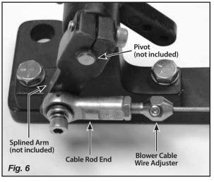
Step 10: At the engine end of the Blower Drive Throttle Cable, slide the blower cable wire adjuster you removed earlier onto the end of the inner wire, all the way up to the throttle cable adjuster. Cut off the inner wire approximately 1/2" away from the splined arm. Slide the blower cable wire adjuster back out to the end of the inner wire and snug down the set screw. Install the cable rod end onto the blower cable wire adjuster. Fig. 6
