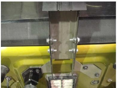
2. Bolt the third brake light mount to the mounting tabs. Use the four (4) 5/16" x 1" bolts to achieve this. Tighten the bolts on the rear door first. Then adjust the mount so that it is straight up and down and tighten those bolts as well.
