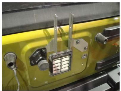
1. If you already have a rear bumper installed you need to start by removing the isolator mount on the rear door. The 3<sup>rd</sup> brake light tabs need to be bolt underneath the isolator mount. Otherwise, begin with mounting the two brackets to the door using the top holes from the factory tire mount. Leave these brackets loose until the next step is complete.
