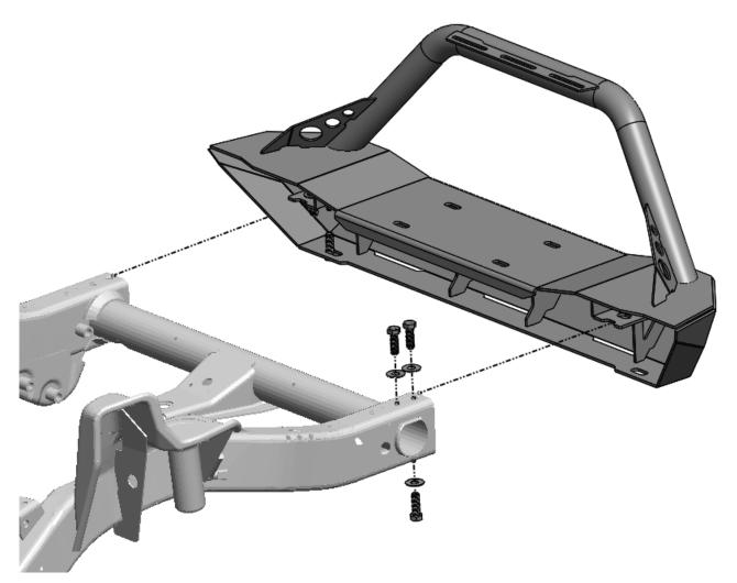
Mount your Destroyer Front Bumper to the original mounting locations on your frame using the provided hardware. If you are installing a winch, do this before mounting your bumper on the frame.
