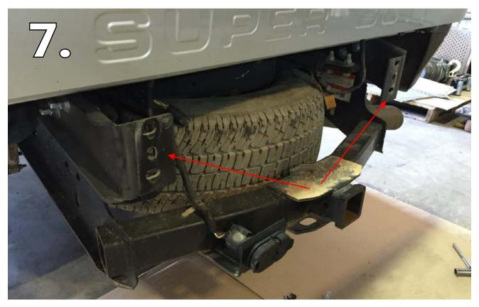
Ready the lod bumper for installation. It is helpful to use a rolling pallet jack to align and hold the bumper during the mounting process.
