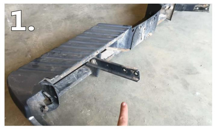
Remove the oem rear bumper, and remove the mounting bolts and brackets underneath the factory bumper.
