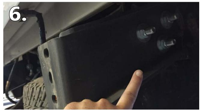
Install the replacement rear mounting brackets on the driver and passenger sides of the frame. use the three 1/2" bolts and nuts provided as shown.
