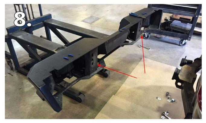
With the bumper ready, align the mounting holes in the bumper and frame mounting brackets. Use the mounting bolts provided in the kit to hold the bumper. leave these slightly loose so the bumper can be leveled before final tightening.
