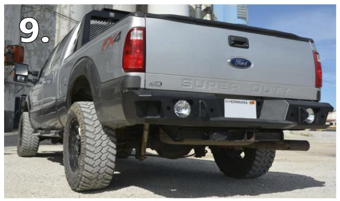
With mounting bolts hand tight, center the bumper to the vehicle. Use a tape measure to confirm that each side has the same amount of overhang and spacing to the vehicle body.
