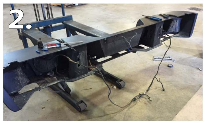
Remove the wiring harness from the oem bumper and place in the LoD bumper
