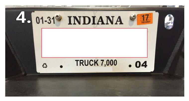
Use the led light bolts to fasten the license plate on the rear bumper pointing the LED lights downwards.
