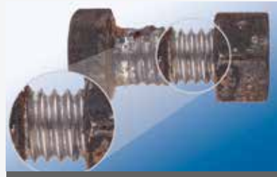
Engagement area of rusty bolt that DID have LOCTITE® threadlocker applied.
