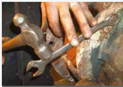
Corroded assemblies can be difficult to take apart...
