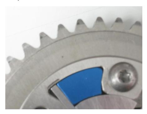
12. The torque for the bolts is 145 in lbs. We recommend using a small dab of blue thread locker on each bolt.
