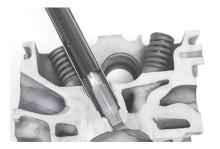
2. Use 3/8" square drive and turn assembly clockwise. Make sure Drill/Tap starts in hole properly and is not angled so hole is drilled properly. Narrow threaded end will pull drill and tap into the head. Make sure to fully tap the new hole.
