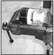
The Handy Packer can be used in a vise with heavy grease. The ribs on the bottom of the cup fit on each side of most vise jaws to hold the cup in place when tightening.
