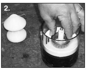
To pack a bearing and remove old grease: Place the bearing with the small taper down over the stem on piston. Put cap on to center bearing. There is no need to screw the cap on to the piston to pack bearings.
