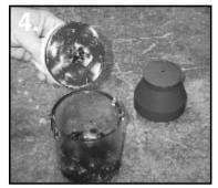
When the cup is empty, screw threaded pusher cap on to stem of piston. Press down and release. The compression spring on the piston helps break the vacuum. Unscrew pusher cap to allow air to enter through piston holes. Screw cap back on to stem and pull assembly to remove from cup to clean or refill.
