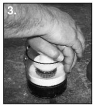
Place the Handy Packer on a flat, solid surface and press down on the cap until the old grease is forced out and new grease shows on top of the bearing.
