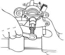
for the car you are servicing. For the counter-clockwise rotation the 1" Hex Nut must be turned more times at a faster rate of rotation in order to keep the adapter engaged with the piston.
