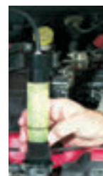
LEAK DETECTED (FLUID CHANGES TO YELLOW COLOR)
