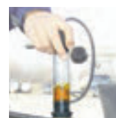
LEAK DETECTED (FLUID CHANGES TO YELLOW COLOR)
