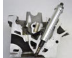
PULLING BROKEN PLUG
