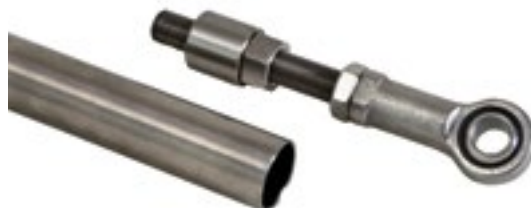
Draglink complete with rod end
