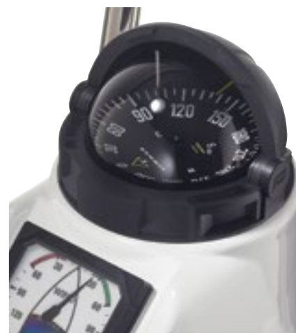
Lewmar 135 Compass flush mounted in pedestal
