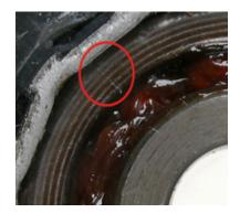
The ball bearing installed in the suspension strut support mount may appear to be moving roughly when it is turned. This is due to the cracking of the outer ring during production and impairs neither function nor service life of the ball bearing.
