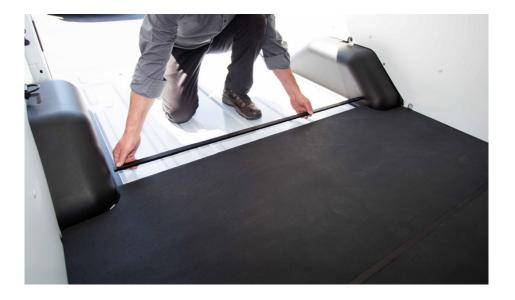
6. Attach the third floor piece (usually the largest) to the rail joint - use a rubber mallet so both floor pieces are secured tightly together.
