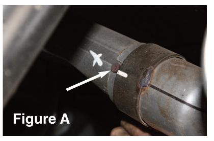
To fit 2007-'11 Jeep Wranglers, the pin (see arrow) on the stock pipe must be removed. Pin is easily removed with a hammer and chisel. Note this pin serves a purpose on the stock exhaust but is not required to install the Legato Performance Exhaust System.
