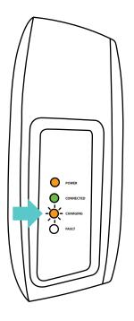
5. When the vehicle is fully charged, the Charging Indicator light will stay solid. Your vehicle has a "dashboard gauge" which can verify that the vehicle is fully charged. Refer to the vehicle owner's manual to find the location of the gauge on your dashboard.
