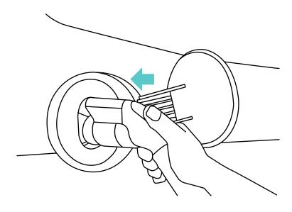
4. Charging begins automatically. Power will be delivered in accordance to the demand of the vehicle. While chaging, the Charging Indicator will blink continuously. Always verify that the vehicle charging status indicator by checking your vehicle panel.
