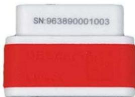
Fig. 1-4 GOLO diagnostic connector (optional)
