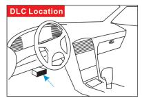
Connect the diagnostic cable into the vehicle's DLC socket.
