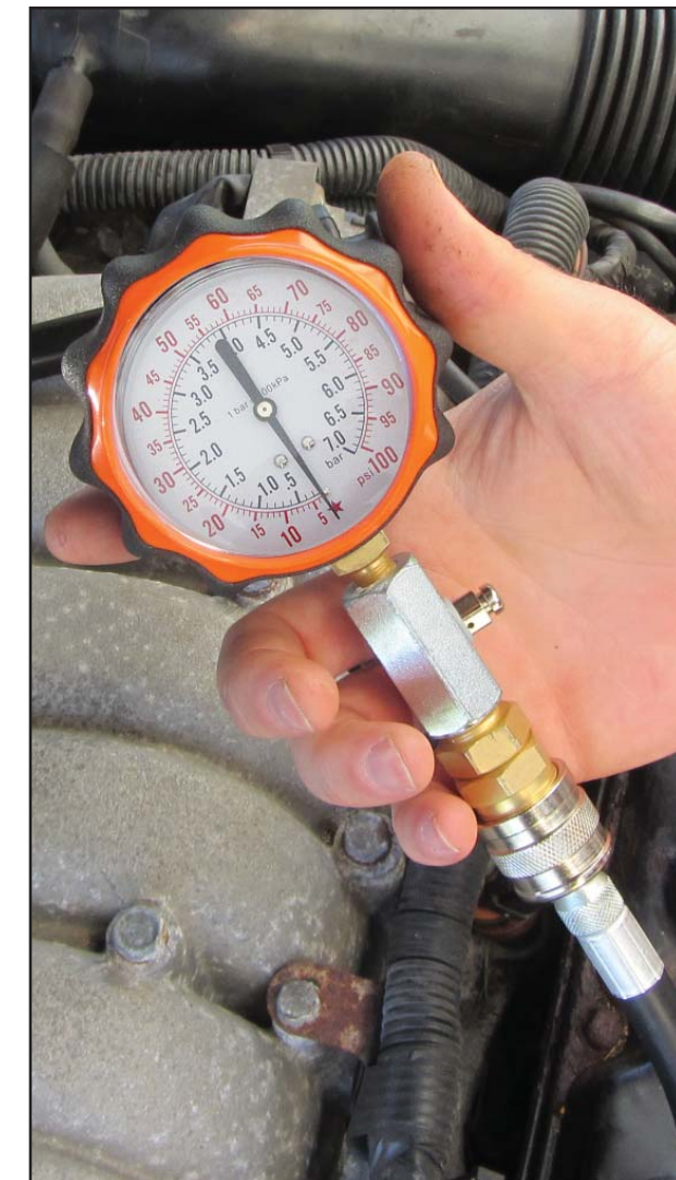
74427: Gauge Assembly on the TU-30A
