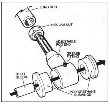
2. Apply lubricant to polyurethane bushings and steel sleeves, then install into eyelet ends as shown.
