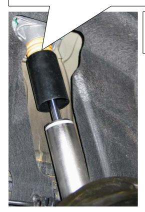
Mount the supplied height adjuster without rubber support between the body and the upper end of the spring.
