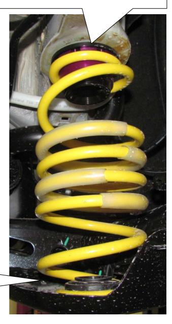
Use the original spring support at the bottom end of the spring.
