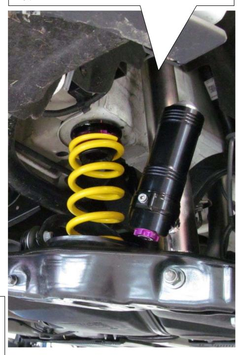
On damper versions with separate reservoirs, mount the reservoir facing to the rear outside of the vehicle as shown on the picture.
