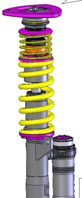
Tightening torque for the top fixing points is 25 Nm (18 ft-lb). The strut unit has to be installed according to manufacturers recommended settings regarding tightening torque and fixing specifications.
