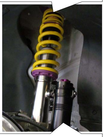
On damper versions with separate reservoirs, mount the reservoir facing to the front of the vehicle as shown on the picture.
