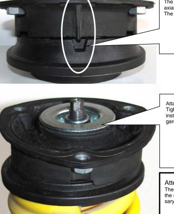
The marks of the OEM upper top mount (upper part) and the OEM axial bearing (bottom part) need to be put on top of each other! The marks show to the vehicle internal side in installed condition.
