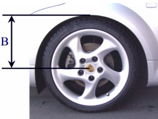
Measurement B Wheel hub center wheel arch
