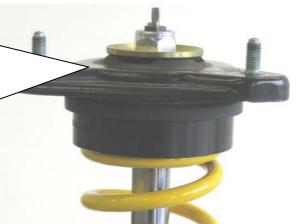
On damper versions with compression balancing case, mount the case in the position to the front side as shown on the picture.
