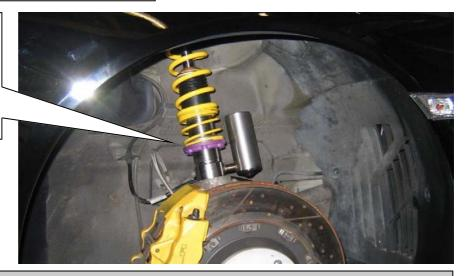
After you have completed installation of the suspension, check the clearance of the tire to the front suspension strut. The minimum clearance at the narrowest point is 5 mm and must, where necessary, be provided using commercially available, Technical Inspectorate (German TUEV) approved spacers.
