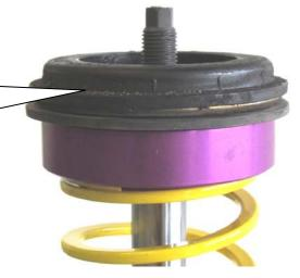
Install the factory top mount and secure it with the supplied nut. Tightening torque for the piston rod is 50 Nm (37 ft-lb). Please install the strut unit to manufacturers recommended settings regarding tightening torque and fixing specifications.
