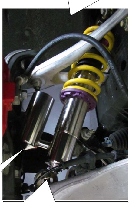
On damper versions with separate reservoirs, mount the reservoir facing to the outside of the vehicle as shown on the picture.
