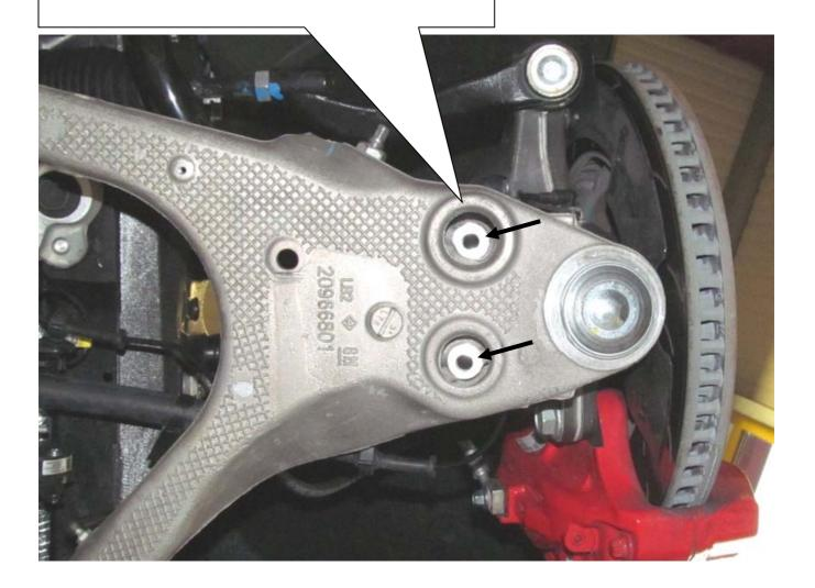
After you have completed installation of the suspension, check the clearance of the tire to the front suspension strut. The minimum clearance at the narrowest point is 5 mm and must, where necessary, be provided using commercially available, Technical Inspectorate (German TUEV) approved spacers.
