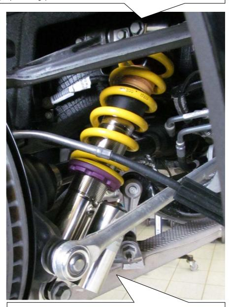
On damper versions with separate reservoirs, mount the reservoir facing to the rear of the vehicle as shown on the picture.
