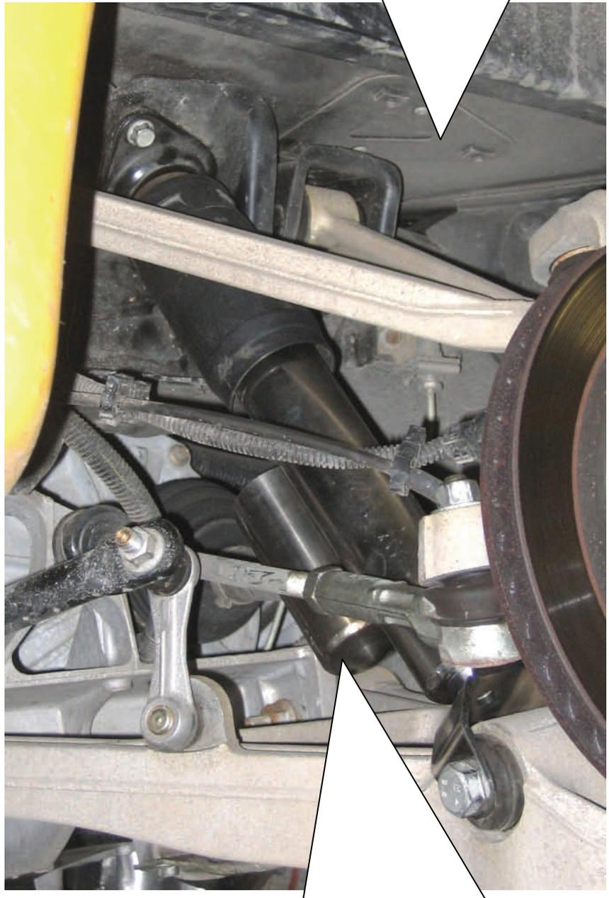
On damper versions with separate reservoirs, mount the reservoir facing the inside of the vehicle as shown on the picture.
