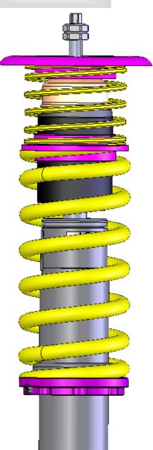
Install the factory supporting bearing and fix it with the supplied nuts. Tightening torque for the piston rod nut is 20 Nm (15 ft-lb). The strut unit has to be installed according to manufacturers recommended settings regarding tightening torque and fixing specifications.
