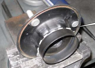
Grinding bottom side to an even surface protected against rust.
