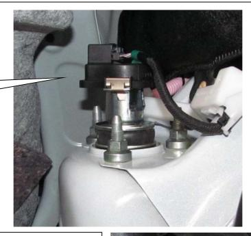
Mount the supplied height adjuster without rubber support between the body and the upper end of the spring.
