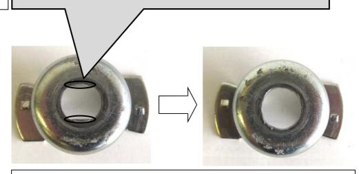
Mount the support bearing from the production car on the supplied suspension strut. In vehicles with electronic damping control, the holder must also be installed too. Tightening torque for the piston rod is 35 Nm (26 ft-lb). Please install the damper unit to manufacturers recommended settings regarding tightening torque and fixing specifications..
