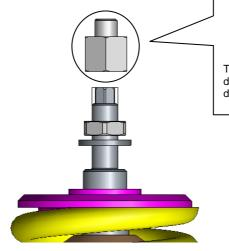
This nut is only required for cars with electronic damping control. For vehicles without electronic damping control, the nut is not required.
