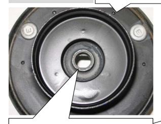
Drill or file out the hole for the piston rod.
