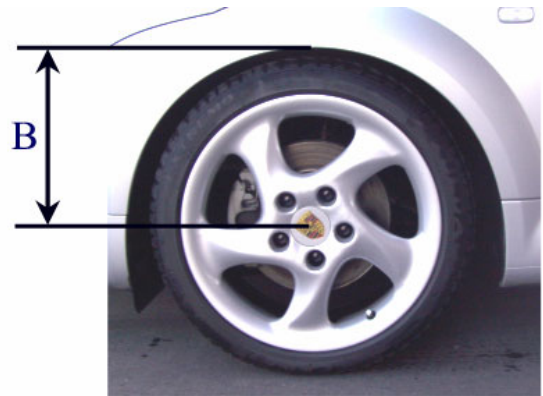
Measurement B Wheel hub center wheel arch
