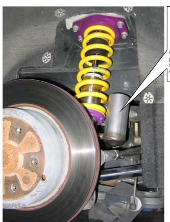
On damper versions with compression balancing case, mount the case in the rear siden as shown on the picture. Insert the standart cover.
