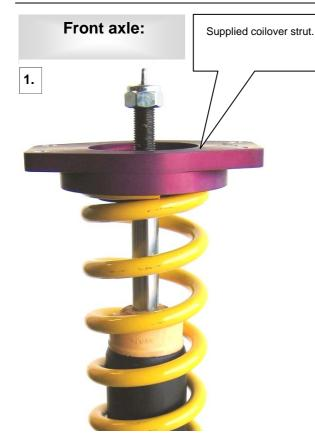
Insert the original gum and mount it with the supplied stop nut. Tightening torque for the piston rod is 60 Nm (44 ft-lb). Please install the strut unit to manufacturers recommended settings regarding tightening torque and fixing specifications.
