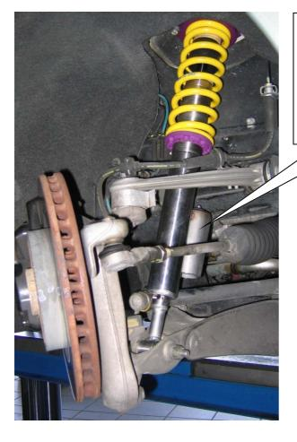
On damper versions with compression balancing case, mount the case in the inside position as shown on the picture. Insert the standart cover.
