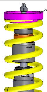
Install the factory top mount without the standard spring perch and secure it with the supplied stop nut. Tightening torque for the piston rod nut is 40 Nm (29 ft-lb). The strut unit has to be installed according to manufacturers instructions settings regarding tightening torque and fixing specifications.
