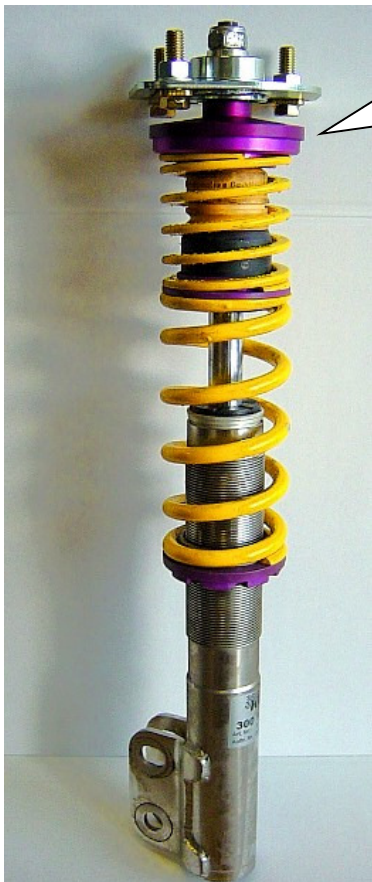
Completely pre-assembled KW coilover strut.
