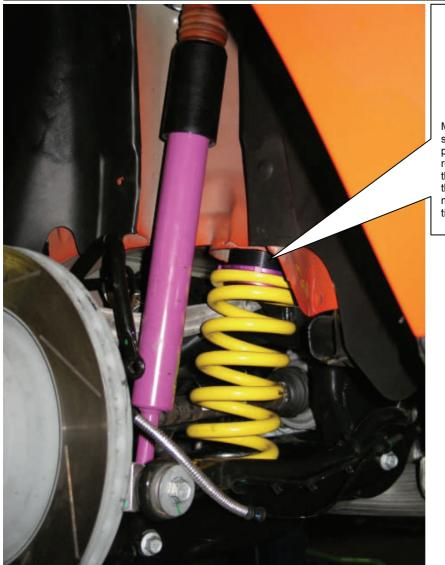
The rear axle shock absorber according to the car manufacturer installation instructions. Unless there is no bump stop in the delivery contents, the standard bump stop has to be used. The standard bump stop has to be in a good condition, otherwise it has to be replaced.
